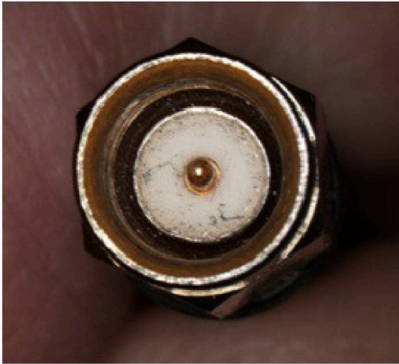
Figure 4. Contaminated SMA connector [2]
