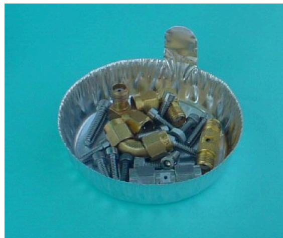
Figure 3. Incorrect way of storing connectors [5]
