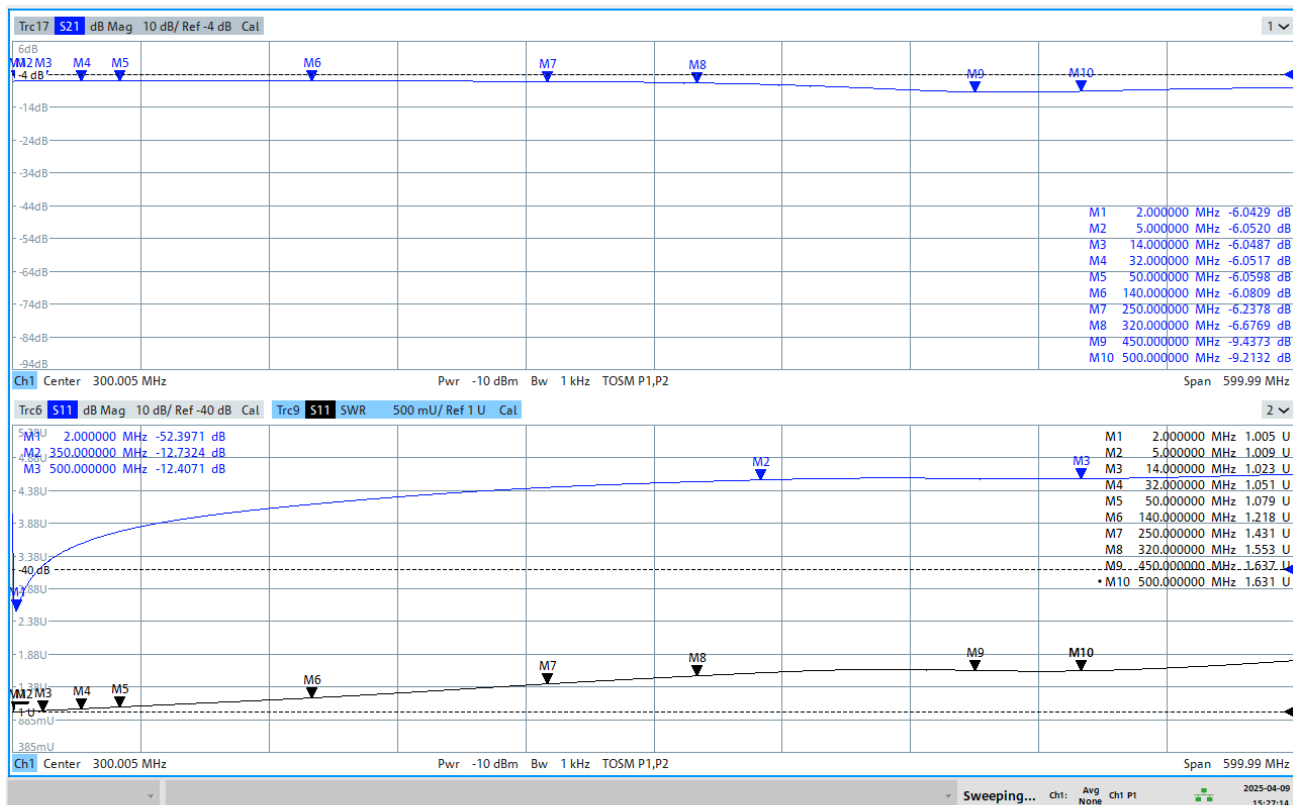
Fig.5 Insertion loss S21 at port P1(A) for RHCS2-6-40C combiner/splitter vs. VSWR (RL/S11)
