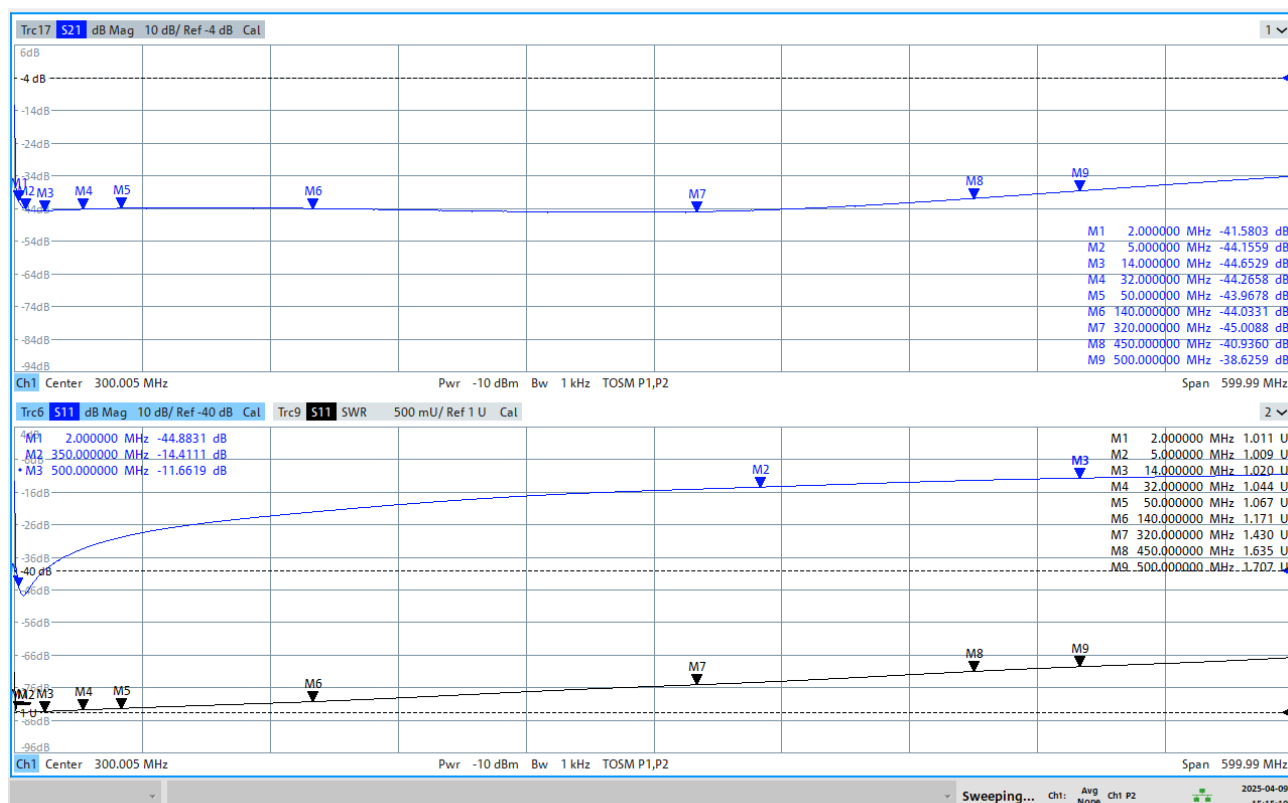
Fig.1 Port-to-port isolation (S21) for RHCS2-6-40B combiner / splitter vs. VSWR (RL/S11)
