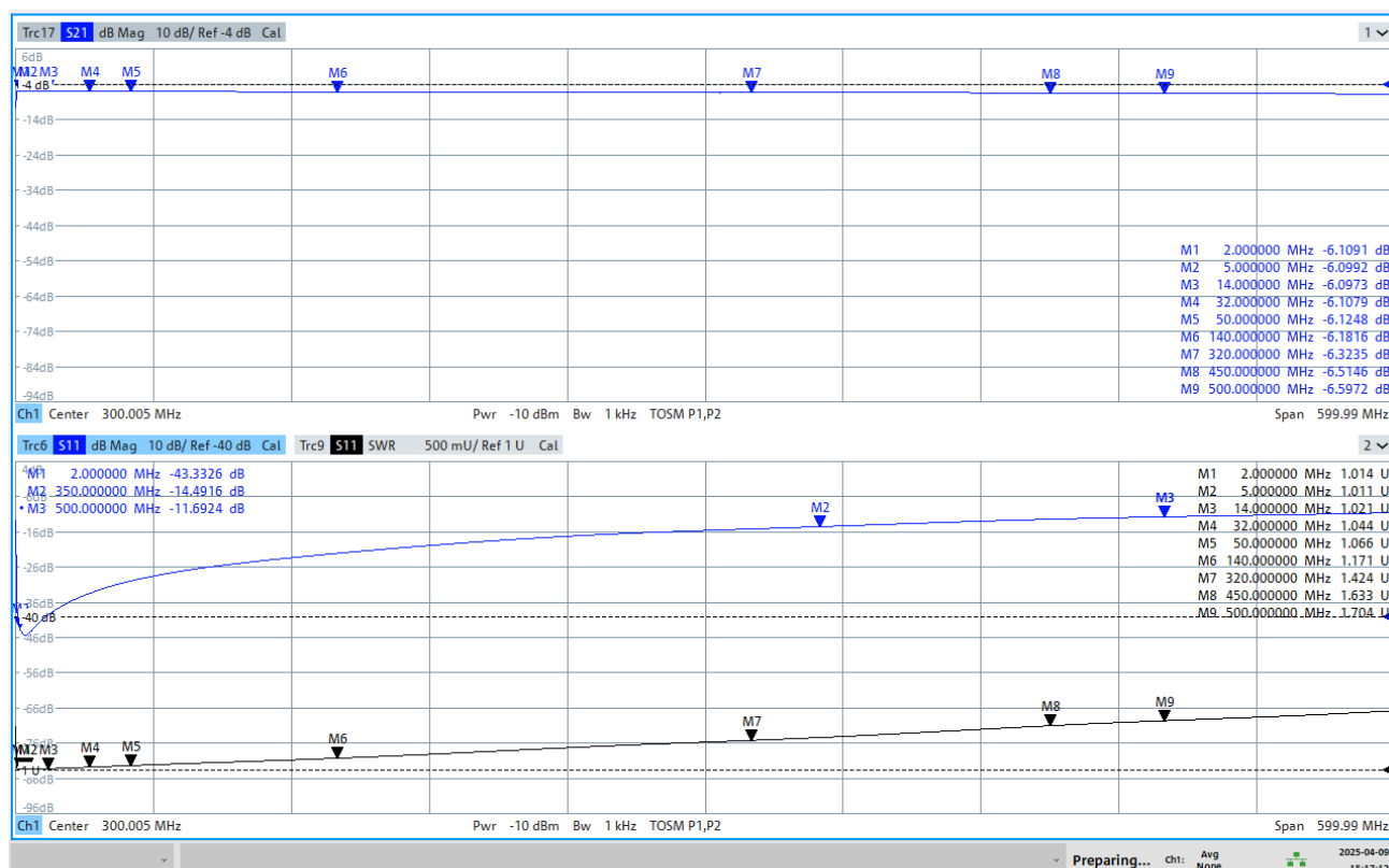
Fig.2 Insertion loss S21 at port P1(A) for RHCS2-6-40B combiner/splitter vs. VSWR (RL/S11)
